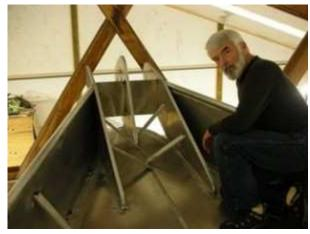
seams are being welded in the proper sequence – the vertical butt seams first and then the longitudinal butt seams; working from the middle of the boat towards each end and also from the chine to the rail and from the chine to the keelson. The last longitudinal welds to be made will be the bottom plates to the keelson and then the topside plates to the rub-rail.
